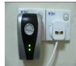
(b) Capacitor connected in socket plug
